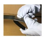
② Pass the end of the strap through in the seal.
