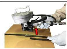
Move the tool in the arrow direction and remove from the strap. The binding is completed.
