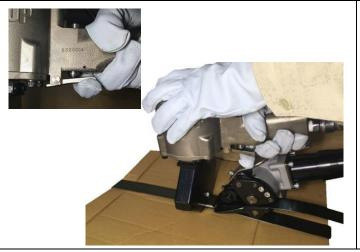
Place sealer over seal, press valve button. After sealing operation is finished, release valve lever and remove sealer from the seal.
