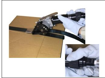
Turn throttle valve counterclockwise. (Feed wheel rotates by air motor) Tightener fastens the strap and holds correct tension on it.
