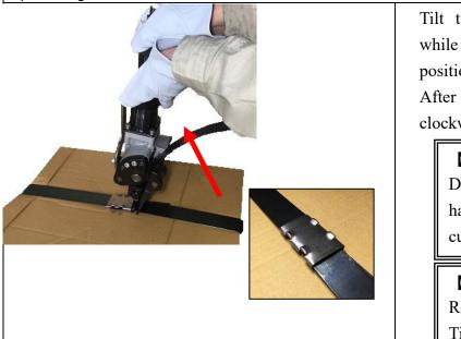
Tilt tightener upward to vertical position while keeping throttle valve at full open position.
