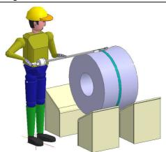
① Direct this tool perpendicular to the strap to cut.
