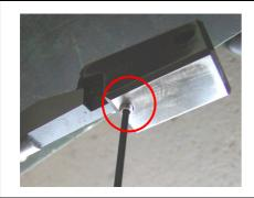
① Remove the M5 hexagon socket set screw from the underside of the gripper.
