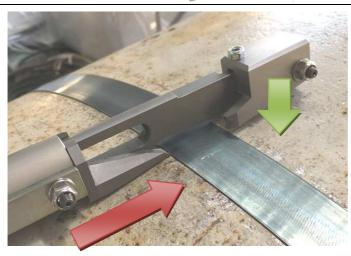
② Run the tip of the knife against or into the end face of the strap.
