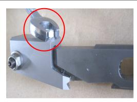
2 Loosen the nut, and turn the gripper angle adjustment bolt to make an adjustment.Tightening the bolt raises the position of the gripper tip, and loosening it lowers the position.
