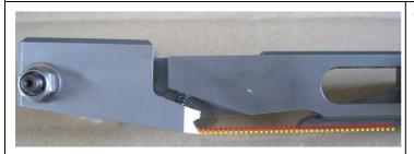
①Before a cutting test, check the coil contact surfaces of the gripper and knife (fixed).
