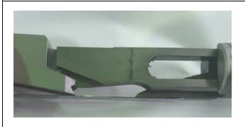
4 As the bolt is fixed with a hexagon wrench to prevent it from being displaced after adjustment, tighten the nut to fix the position of the gripper.
