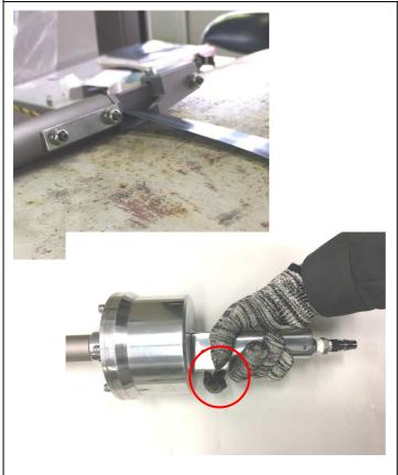
4 While holding the cutter in a set state, push the valve button with your index finger to cut the strap.
