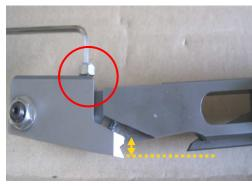
③ Tighten the bolt to make an adjustment so that it becomes parallel to the knife tip.
