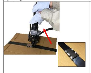
Tilt tightener upward to vertical position while keeping throttle valve at full open position.
