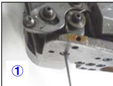
① Remove a hexagon socket head screw with a 3mm hexagon wrench.
